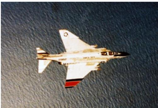
The Phantom was one of the first fighters adopted by multiple armed services. Developed for the U.S. Navy, the F-4B was compared with Air Force fighters in 1961 and found to out-perform all by a wide margin. The two-seat Phantom flew at 1,500 mph (2,415 kph) at heights up to 50,000 feet (15,239 meters). More than 5,000 were produced and flown by American and foreign armed forces.
