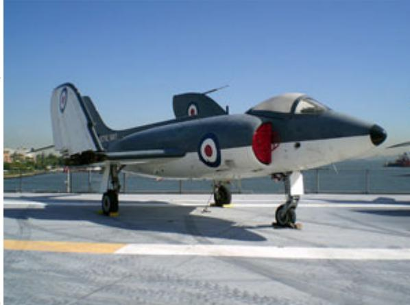
In contrast to its predecessors, the Scimitar utilized an area-ruled fuselage, the distinctive “Coke-bottle” shape that reduces drag at high speeds. This helped the aircraft fly at speeds up to 710 mph (1,145 kph) and heights up to 50,000 feet (15,200 meters). This type of fuselage was pioneered by American scientist Richard Whitcomb. The Scimitar had a short career with the Royal Navy and flew in NATO exercises alongside *Intrepid* aircraft. Scimitars remained in service until 1969.
